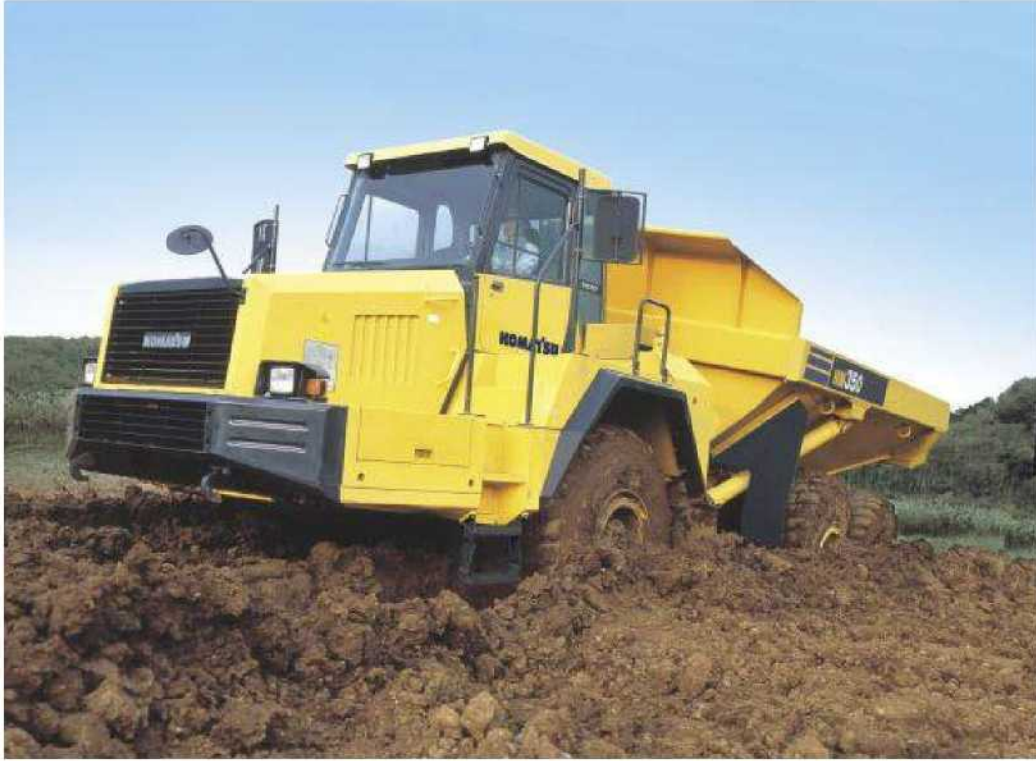
Figure 8-7. Articulated dump truck ( photo courtesy of Komatsu ).
