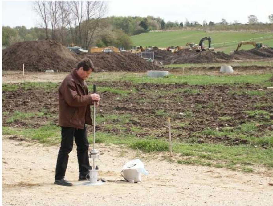
Figure 8-3. Lightweight deflectometer ( photo courtesy of Dynatest ).
