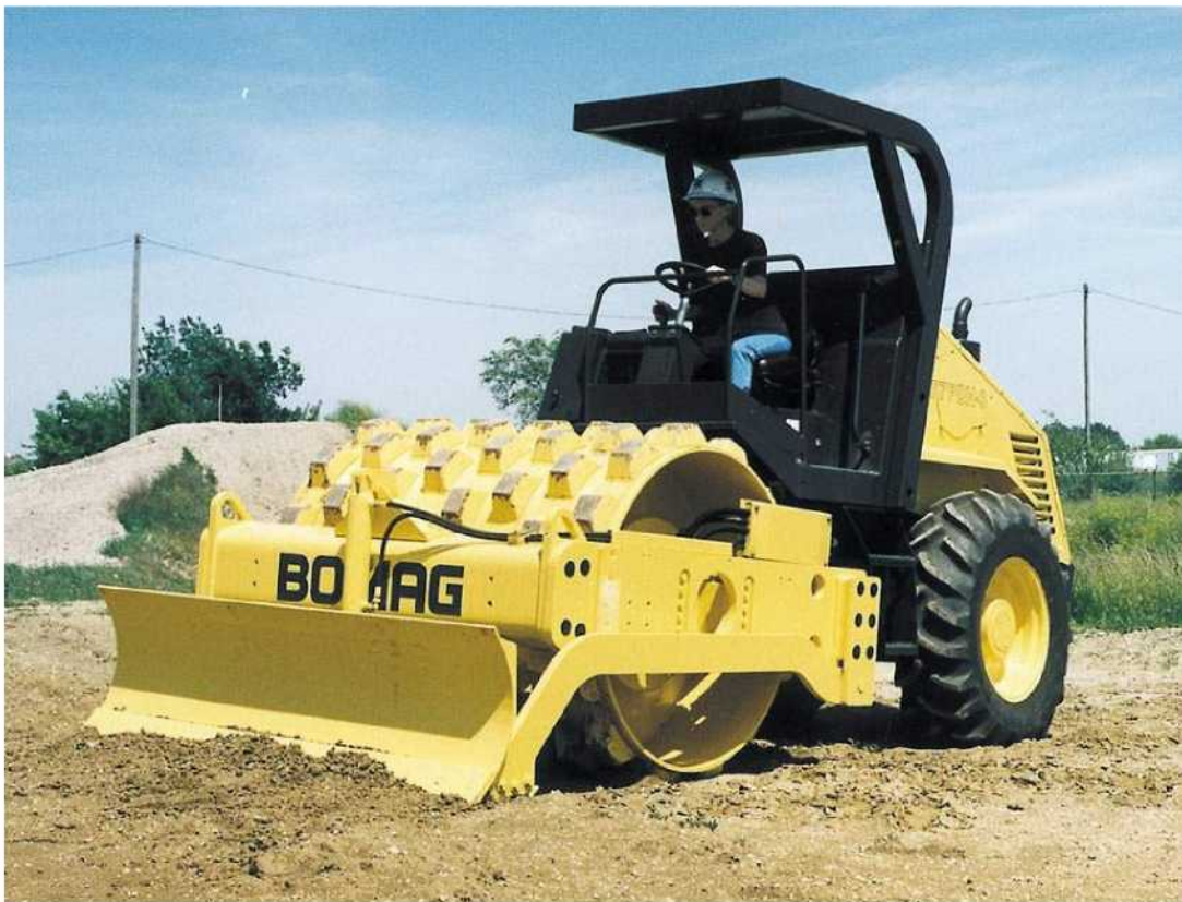
Figure 8-13. Sheepfoot roller ( photo courtesy of Bomag ).
