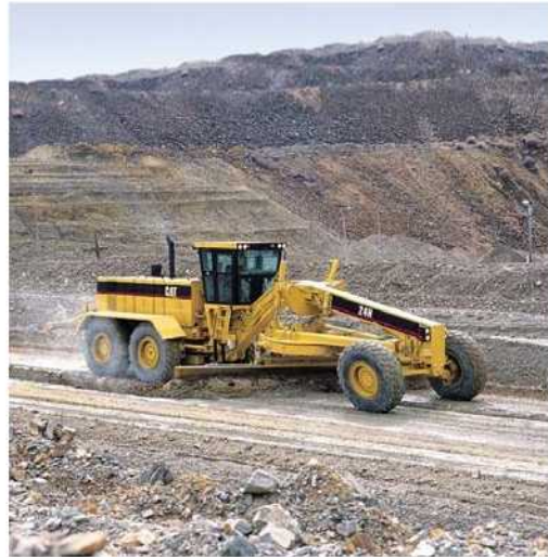
Figure 8-9. Motor grader ( photo courtesy of Caterpillar )
