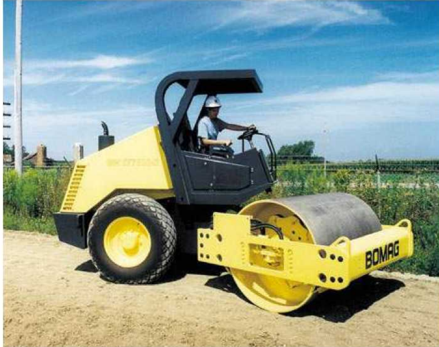
Figure 8-12. Smooth drum roller ( photo courtesy of Bomag ).
