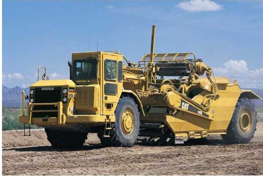
Figure 8-5. Self-loading scraper (photo courtesy of Caterpillar).
