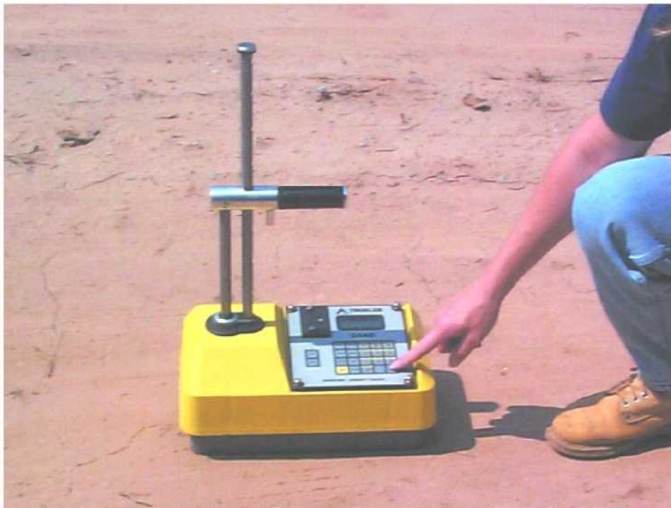
Figure 8-1. Nuclear densometer ( photo courtesy of Troxler ).
